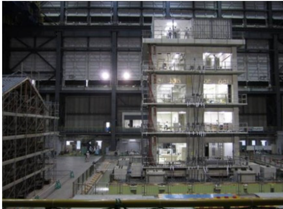
FIGURE 28. Large-scale simulation of a building on an earthquake simulator in Japan
