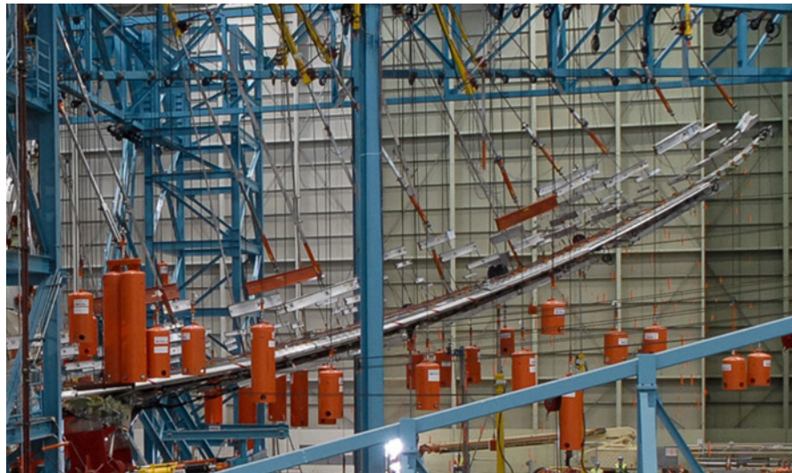
FIGURE 24. Load test on a Boeing 787 Dreamliner wing
